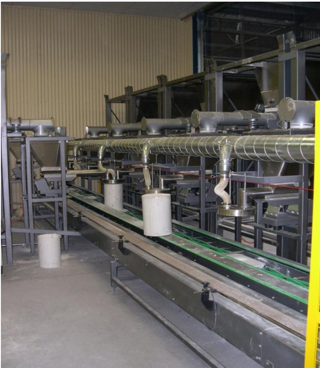
*Shows bag holders travelling down belt conveyor and individual product vibratory filling stations.*
