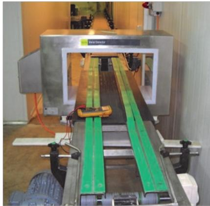
Metal detector implemented onsite at New land Foods. Metal detector model Genie 600/350 Genius +. Implemented into their existing conveyor belt.
